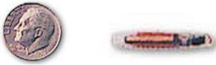
Figure 1. PIT tag (32 mm) shown with a dime coin for size comparison.
